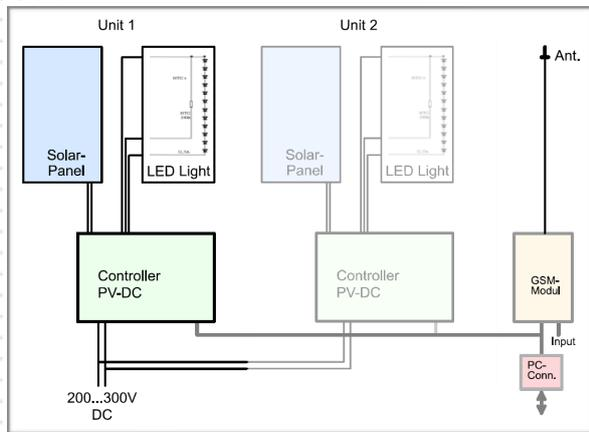
**Power Station type (PS) with option (r) - remote control (GSM module).** Multiple SOLED XP luminaries are connected together via a DC-Bus to deliver energy back to the grid (energy recovery). The SOLED PV-DC controller delivers energy to the DC bus and draws energy from the DC bus.
